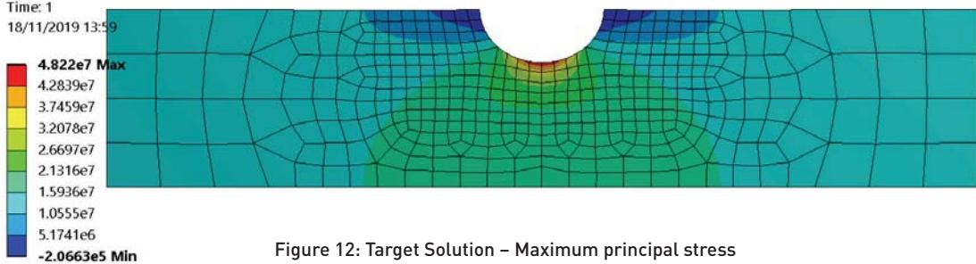
Figure 12: Target Solution – Maximum principal stress
