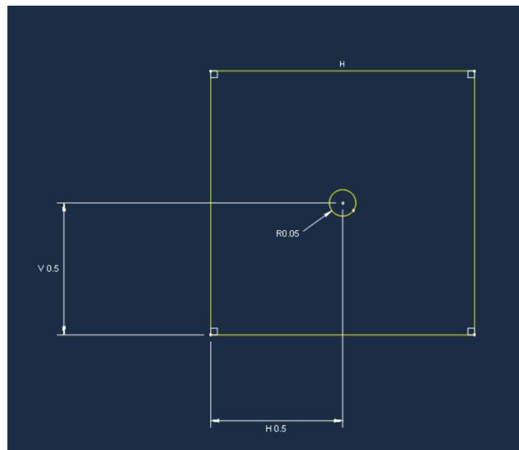
Figure 8: Geometry of the plate with hole benchmark
