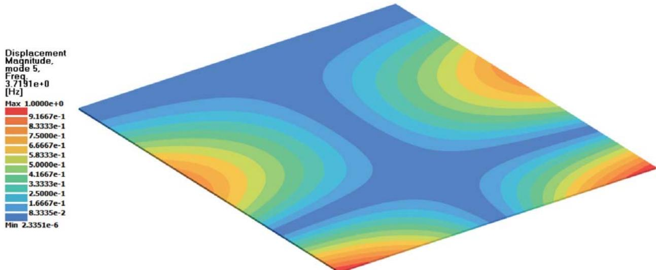
Figure 14: SimSolid - Displaced mode shape – Mode 5 – 3.72Hz – Benchmark 7
