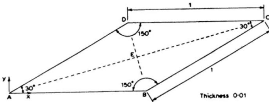
Figure 5: The geometry of the skewed plate
