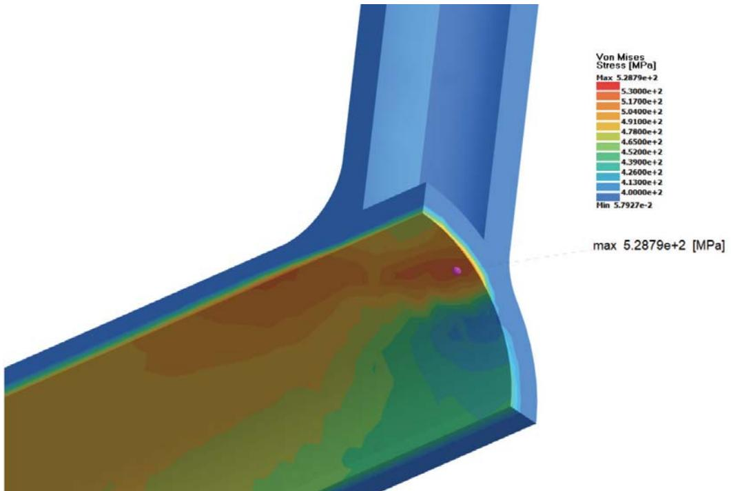
Figure 3: SimSolid - Contours showing Von Mises Stress
