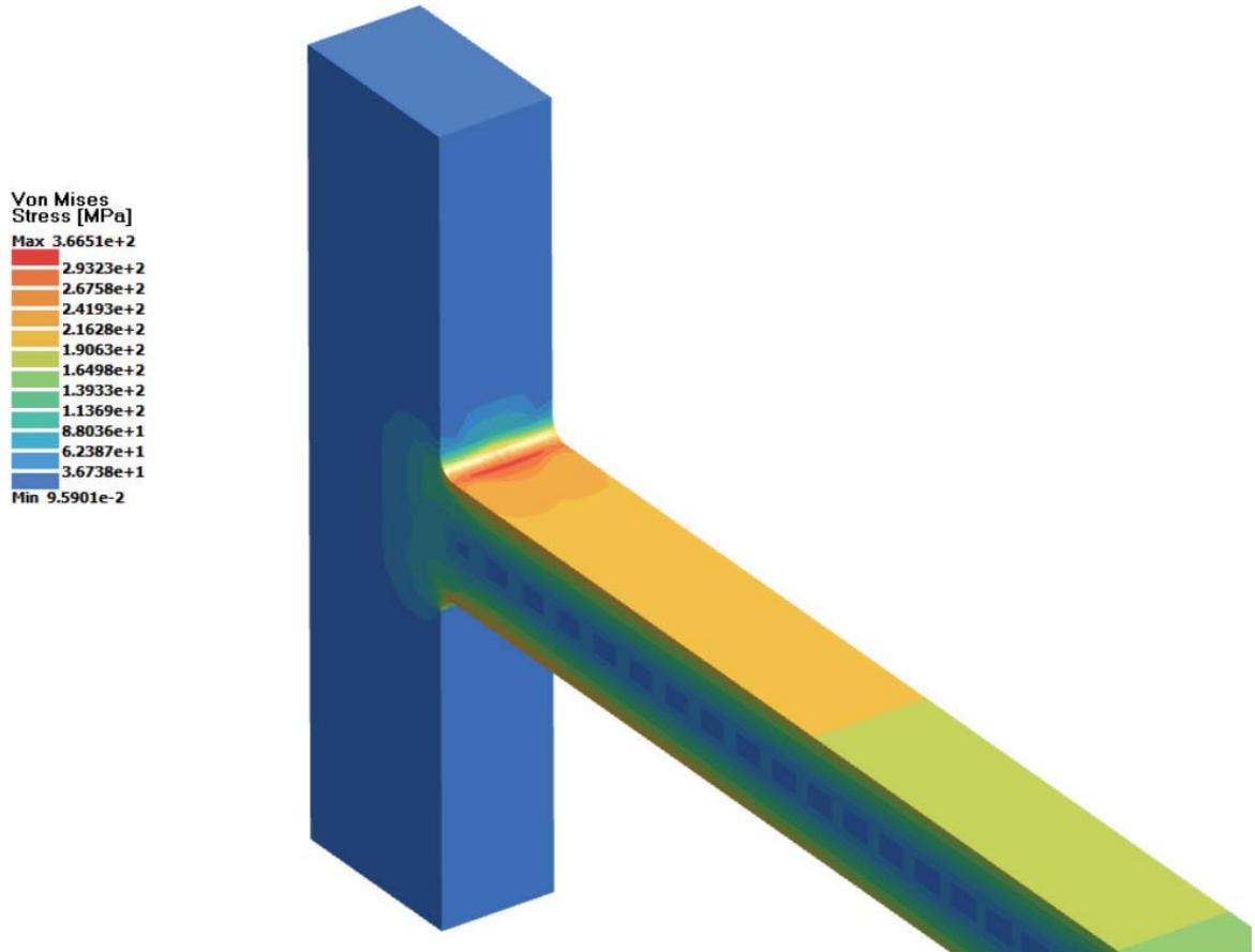
Figure 19: SimSolid – Von Mises Stress
