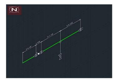
Since the isometric drawing is not to scale, all the dimensions need to be entered. Also, the MTO table must be entered manually as an AutoCAD table, thus requiring a lot of input even for an experienced AutoCAD user.
