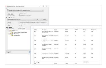
Using basic AutoCAD, this task is usually performed using an Excel spreadsheet. It's a manual task, and designers must check to ensure no items are missing. Also, there is no link between the spreadsheet and the data source, so changes made in basic AutoCAD require a manual update of the spreadsheet.
