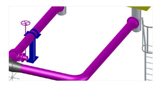
The designer then inserts the valve by selecting it from the spec and identifying the insertion point in the pipe.
