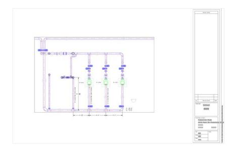
After creating the viewport, the designer can use the Plant 3D toolset 'annotation' commands to add equipment tags, line numbers, piping elevations, etc. The toolset employs standard dimensioning to place linear dimensioning:
