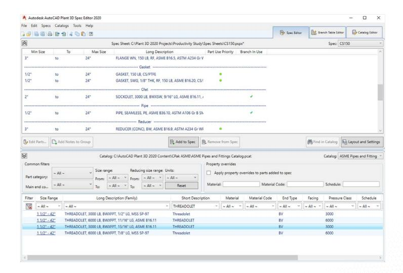
Using the 'Add to Spec' command automatically adds the selected threadolets to the pipe spec. The Plug and nipples are added in the same way.
