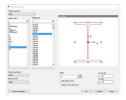
The designer does not need to enter any of the shape dimensions as they are extracted from steel catalogs.
