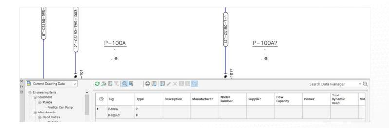
Data Manager allows users to view the data and then export it to Excel using the 'export' command. Once exported, they can edit the data in Excel and then import it back into the Plant 3D toolset using the Data Manager 'import' command. Differences between the P&ID and the Data Manager are highlighted below:
