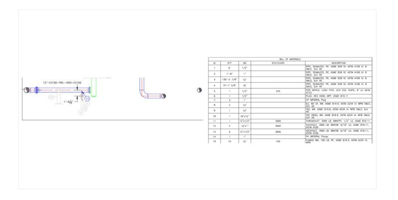
The BOM annotation for the new components (nipple, valve, and plug) are added automatically. The dimensioning must be updated manually.
