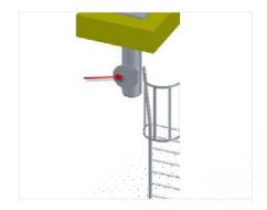
The designer simply selects the 'route pipe' command and selects the pipe route. In this case, the end of the pipe at the reducer and the pump nozzle:
