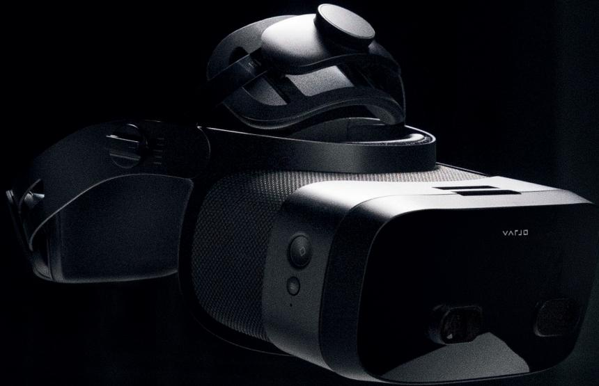
VR-3 and XR-3 feature the world's fastest and most accurate eye tracking at up to 200 Hz, giving users optimized visual fidelity through foveated rendering and enabling analysis of even the smallest eye movements.
