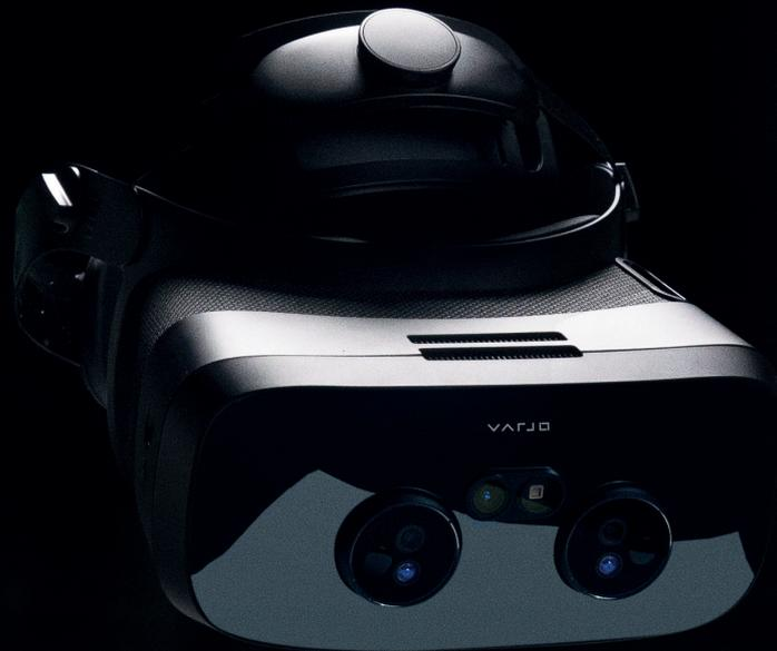
LiDAR and stereo RGB video pass-through deliver seamless merging of real and virtual for perfect occlusions and full 3D world reconstruction.
