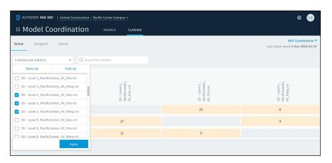
PRO TIP: Search and filter models within the clash matrix (using model naming conventions) to focus review on a specific location. Click on the row header to open and view all models and clashes within that context.
