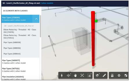
PRO TIP: Users can create groups of clashes using inherent BIM object data depending on the format type (i.e. Revit (RVT), AutoCAD (DWG) and IFC) such as System Name, Layer and Type Name.
