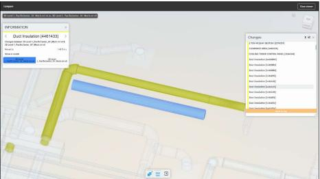
Issues are used by teams to identify and communicate areas of concern or improvement with project documents or models. The BIM 360 Issues workflow is unified into the Model Coordination module. This allows users to view issues across multiple models (i.e. clashes can be assigned to multiple models that the issue is linked to and retains the clash highlighting).
