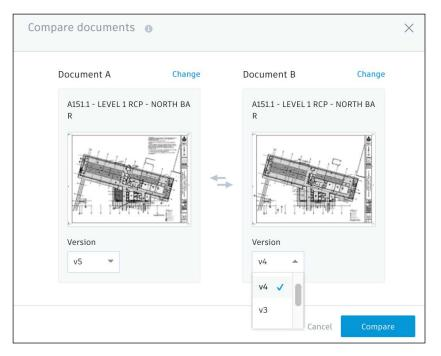
PRO TIP: With 2D compare, you can compare two versions of the same drawing or model or two entirely different drawings. For example, you could compare drawings from two different disciplines.
